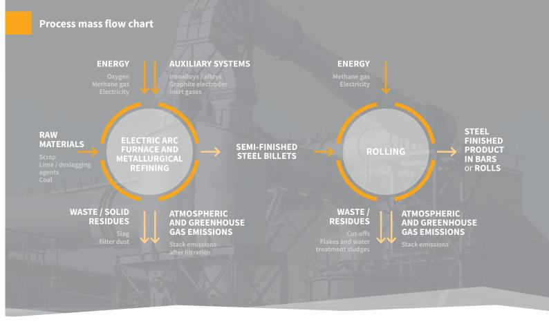
The rolling processes at the aforementioned sites and at **Fer-Par** (Brescia, Italy) must be considered energy-intensive given the high amount of methane gas consumed to heat and process billets into semi-finished and/or finished products.
