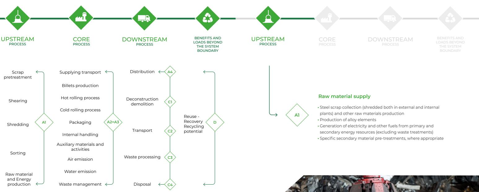
Broad scheme of hot rolled steel production, in which the main activities included in the system boundaries are listed and divided in the three subsystems: UPSTREAM Process, CORE Module and DOWNSTREAM Process.
