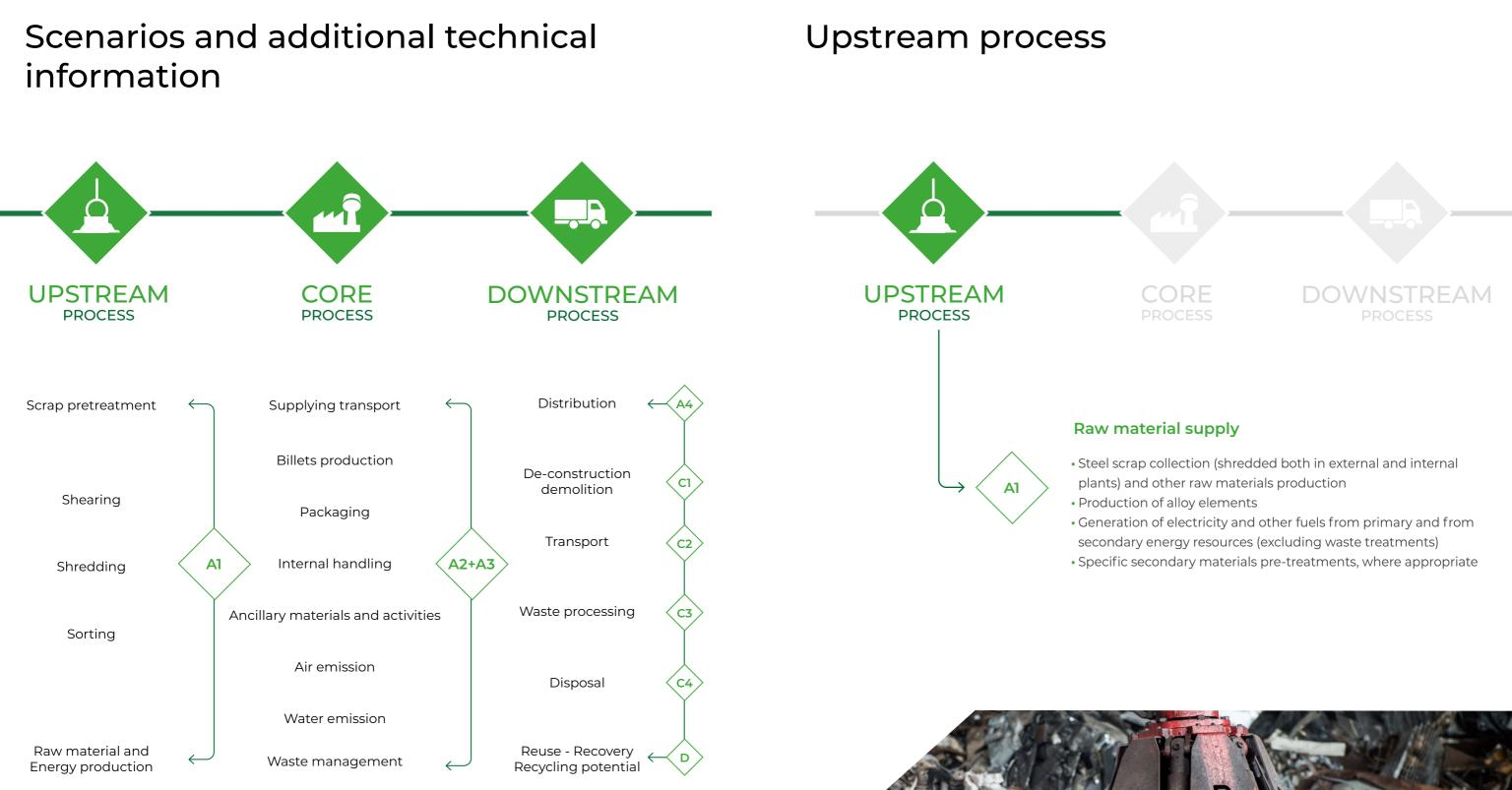
Broad scheme of steel billets production, in which the main activities included in the system boundaries are listed and divided in the three subsystems: UPSTREAM Process, CORE Module and DOWNSTREAM Process.
