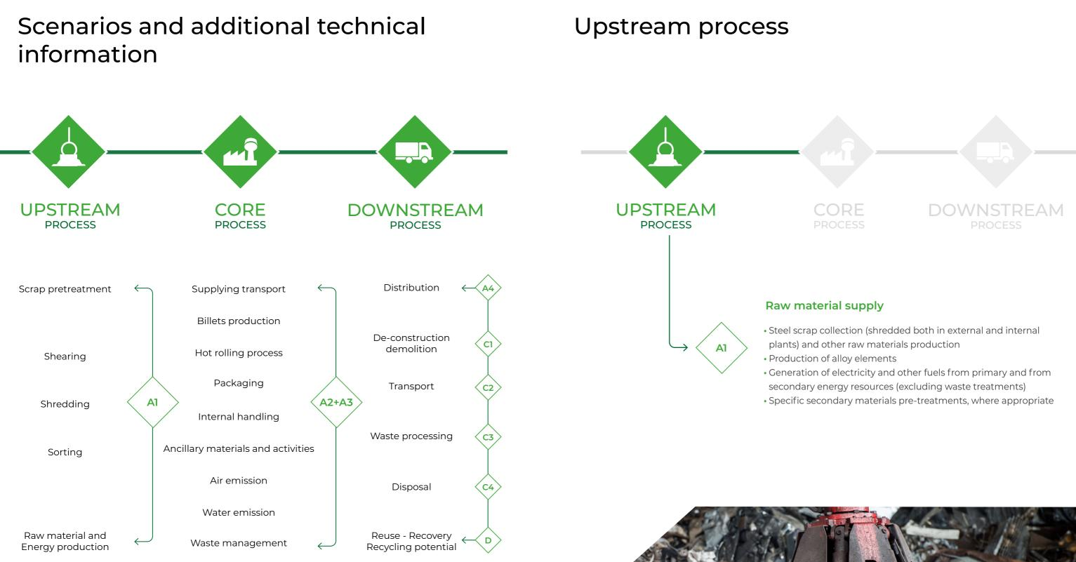
Broad scheme of hot rolled steel production, in which the main activities included in the system boundaries are listed and divided in the three subsystems: UPSTREAM Process, CORE Module and DOWNSTREAM Process.
