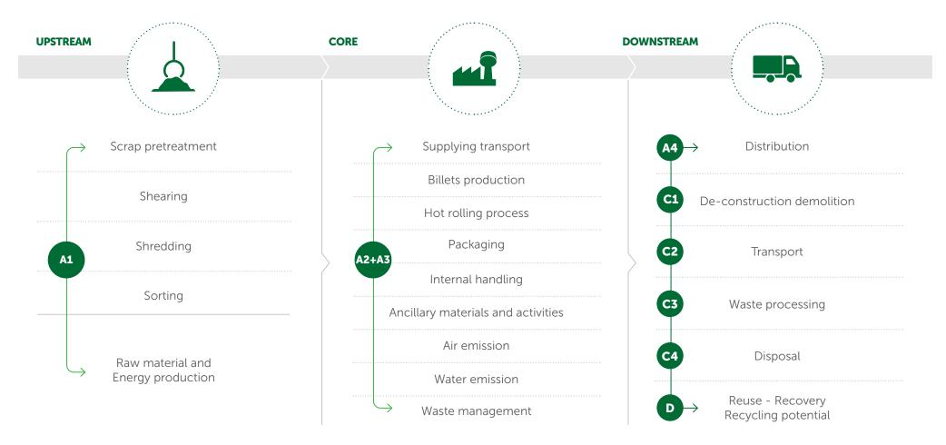
Broad scheme of hot rolled steel production, in which the main activities included in the system boundaries are listed and divided in the three subsystems: **UPSTREAM Process, CORE Module and DOWNSTREAM Process**.
