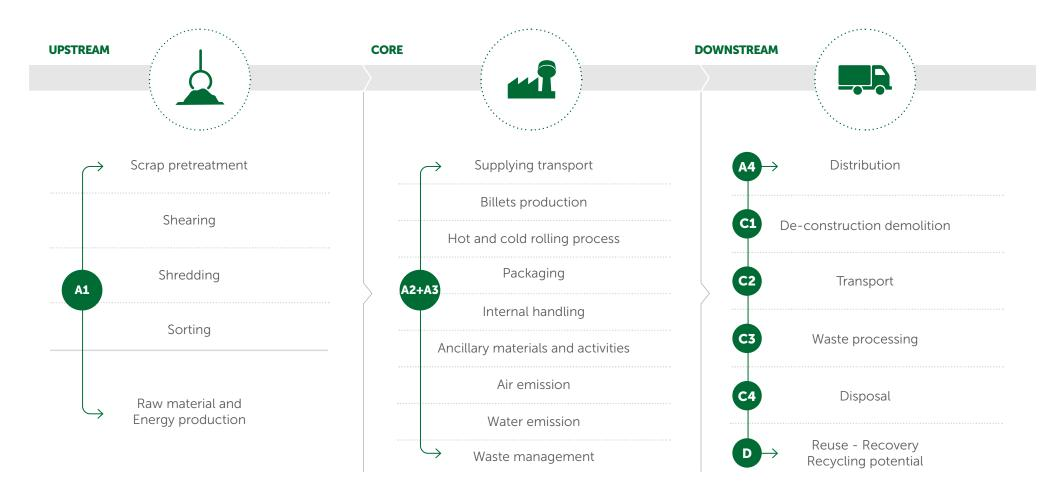
Broad scheme of cold rolled steel production, in which the main activities included in the system boundaries are listed and divided in the three subsystems: **UPSTREAM Process, CORE Module and DOWNSTREAM Process**.
